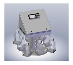
Our design started with a carousel-style bottle holder with the enclosure mounted above. This bi-level approach allowed us to weigh up to eight bottles in a relatively compact space, but bottles in the rear would be difficult for operators to access.
