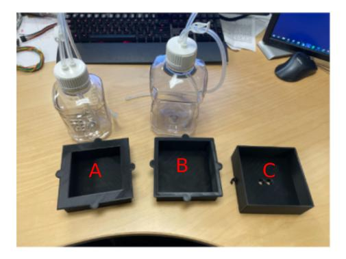
A: This bottle holder inserts into the carrier (C) and holds a 500mL bottle
