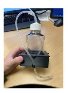
Both bottle holder inserts fit into the same carrier, allowing the operators to quickly and easily change what size bottle they want to feed into their bioreactors. The carriers also feature a clip to secure the tubing to help reduce tubing pulsations from the peristaltic pump and help keep the benchtop space neat.
