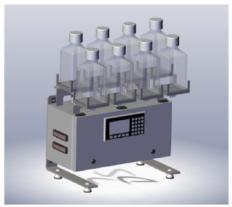
Our second design mounted load cells to the top of the enclosure. This ensure full access to all bottles, but still occupied too much bench space.
