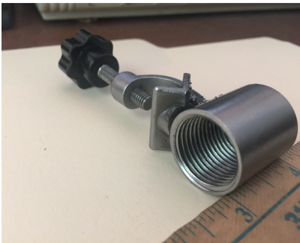
FIGURE 13 - BOSS HEAD MOUNTING CLAMP
